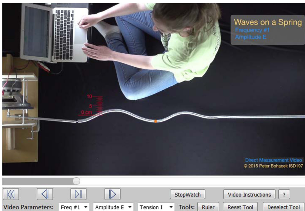
FIG. 1. This video shows a wave moving down a large horizontal spring. Students can access interactive tools by selecting the Ruler and Stop Watch buttons on the bottom toolbar. Using the tools, they can measure the amplitude, frequency, wavelength, period, and speed of the wave. As indicated on the bottom toolbar the current video shows the lowest of five possible frequencies, the largest of five possible amplitudes, and the lowest of three possible tensions. By using the drop-down menus students can select different values for these parameters, which allows them to easily perform a range of experiments. For the model-making assessment (Appendix A), students in classes that had not studied wave phenomena were asked to determine the relationship between the wavelength and frequency of a wave. Successfully completing that task required students to design, execute, and analyze an experiment where the frequency of the wave was varied and the wavelength was measured (while holding the other parameters constant). You may use this online resource for free at the link in Ref. [35].
